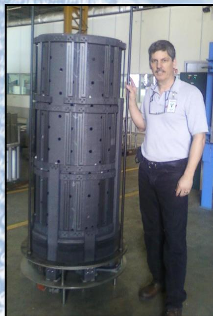
Above: AIP 22" diameter x 60" long Carbon furnace rated for 2000 C.
