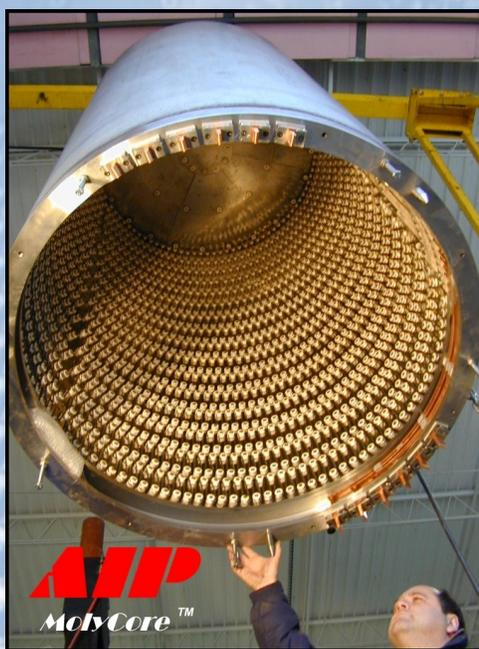
Above: AIP 46" diameter x 80" long Hybrid Inconel-Molybdenum furnace rated for 1225 C. Internal wound for maximum hot zone space.
