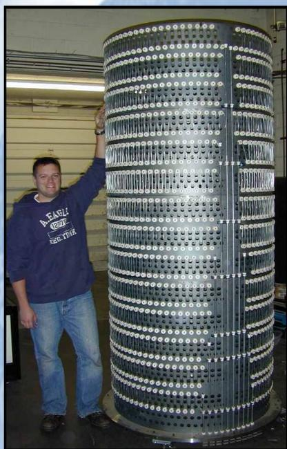
Above: AIP 30" diameter x 80" long Molybdenum furnace rated for 1400 C.
